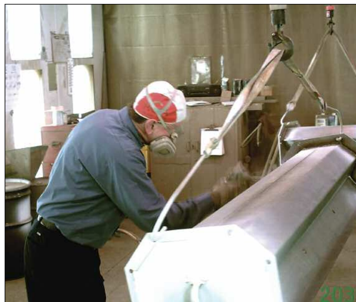
ROY MEEDS of Piqua paints a section of a side wall return drag conveyor trough.
